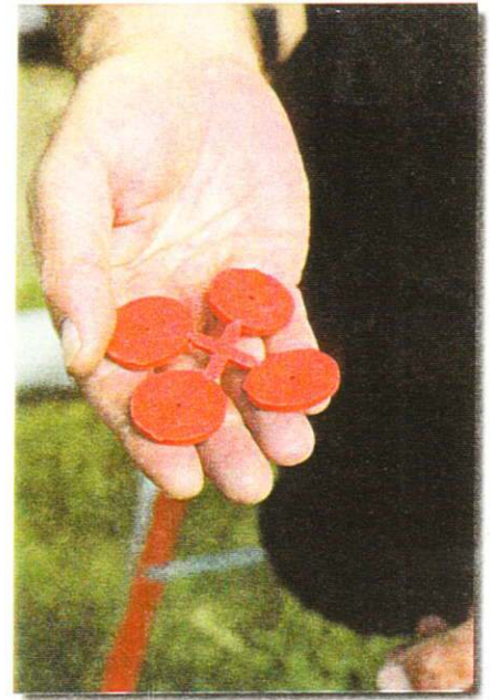
Drainage washer for bottom of first flush diverter.
